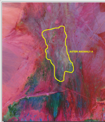
Fig. 5. Improved remote sensing and advanced spectral processing use mineralogical changes to search for potential hydrocarbon seeps.
